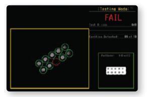
The blisters **expand under vacuum**, driving air out of the blister through any leaks present. If there is a leak in the blister, the **air escapes into the chamber**, leaving a collapsed blister package.
